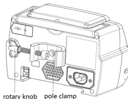
(3) If mounting on pole, rotate the pole clamp screw(knob) and unscrew to leave space. Lock the Pole Clamp on the infusion stand, adjust the position of the infusion pump, tighten the pole clamp to fix the infusion pump on the infusion stand (shown in drawing to the right). Hold the infusion pump when tightening the fixing clamp; loose it after tightening to avoid falling.
