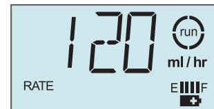
Figure 2-13 Pump is Running
