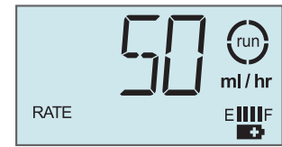
Figure 2-20 Pump is Running
