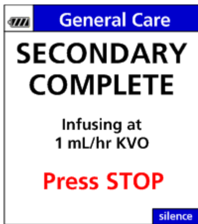
Figure 45. Secondary Completion; KVO Alarm.
