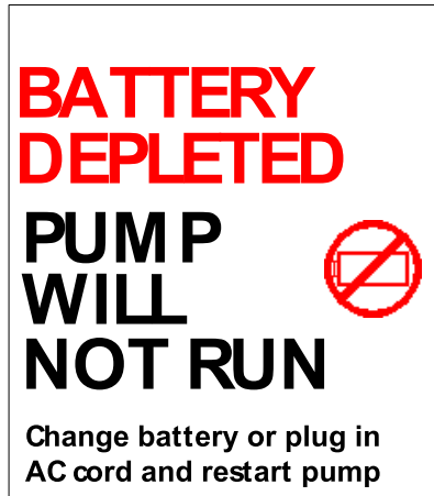
Figure 69. Battery Depleted Alarm.
