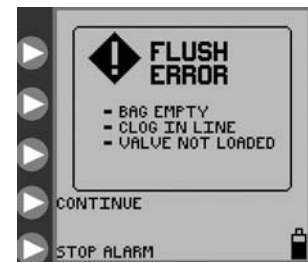
Figure 28. Flush Error screen.
