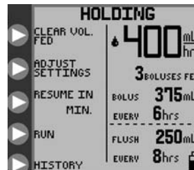
Figure 18B. HOLDING mode options, intermittent feeding mode.
