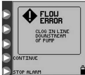
Figure 29. Flow Error screen.
