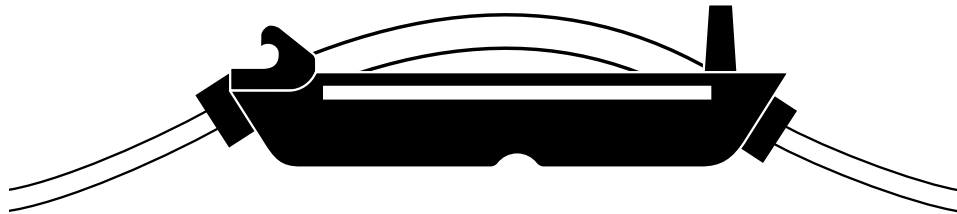
Figure 3. The administration set plate is inserted in the bottom of the pump.
