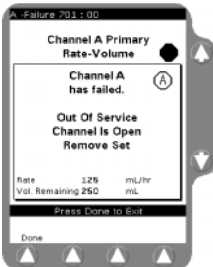
Figure 6-10 Channel Failure Pop-up Message
