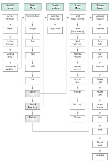
The pump can be customized by (de-)activating the menu itmes of the Start Up- and Options Menu as well as the bolus function via the service program.
