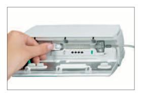
In the next step, attach the white clip without twisting the line. Properly insert the line into the air-sensor.
