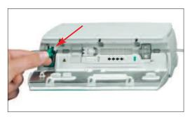
Insert the freeflow clamp (see red arrow) in the opened aperture, in the direction indicated by the arrow, until the opening lever locks in and the safety clamp squeezes the lines (flashing signal lamp goes out).
